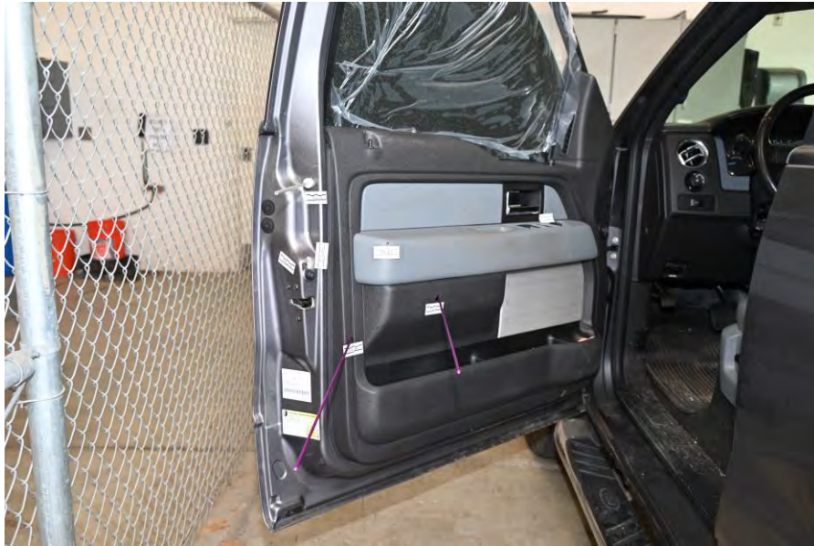
Figure 1: A view of the driver's door interior, showing the ballistic impacts with scales and trajectory rods in place.
