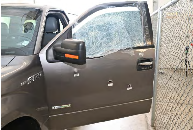
Figure 3: A view of the driver's door exterior with scales and trajectory rods in place.
