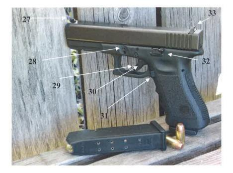
Match the labeled part LETTER to the appropriate number as listed below. 27 28 G 29 F 30 E 31 D32 C 33 B A. FRONT SIGHT **B. REAR SIGHT** C. SLIDE RELEASE LEVER D. MAGAZINE RELEASE E. TRIGGER F. SAFE ACTION TRIGGER SAFETY G. DISASSEMBLY LATCH
