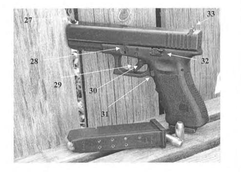
Match the labeled part LETTER to the appropriate number as listed below. A 27 28 G 29 F 30 E 31 D 32 C 33 P A. FRONT SIGHT B. REAR SIGHT C. SLIDE RELEASE LEVER D. MAGAZINE RELEASE E. TRIGGER F. SAFE ACTION TRIGGER SAFETY G. DISASSEMBLY LATCH
