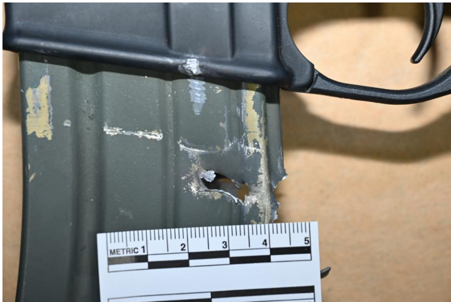
Ballistic impacts observed on the DB15 rifle (Item 33).
