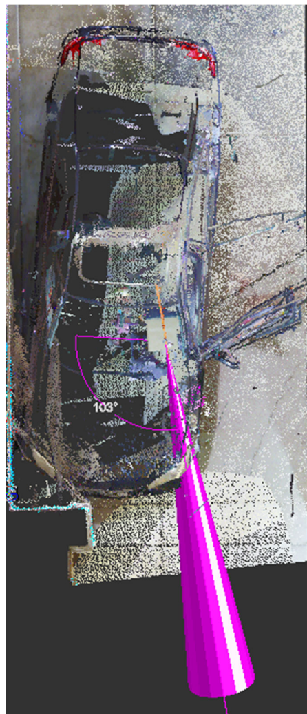
Image 5. 5° trajectory cone of BE 1 into windshield
