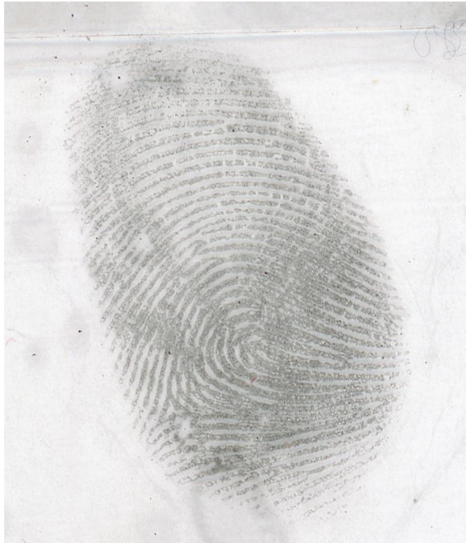
**Second touch (ST) – overlapping impressions of the same ridge detail with complete lift off from surface**
