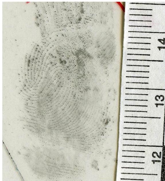
Example: distortion due to pooling of extra matrix (white powdered print)
