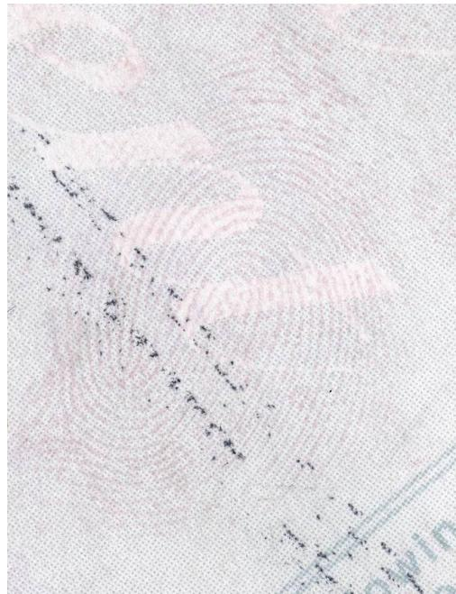
Example: distortion due to textured substrate (powdered print on ridged duct tape surface)
