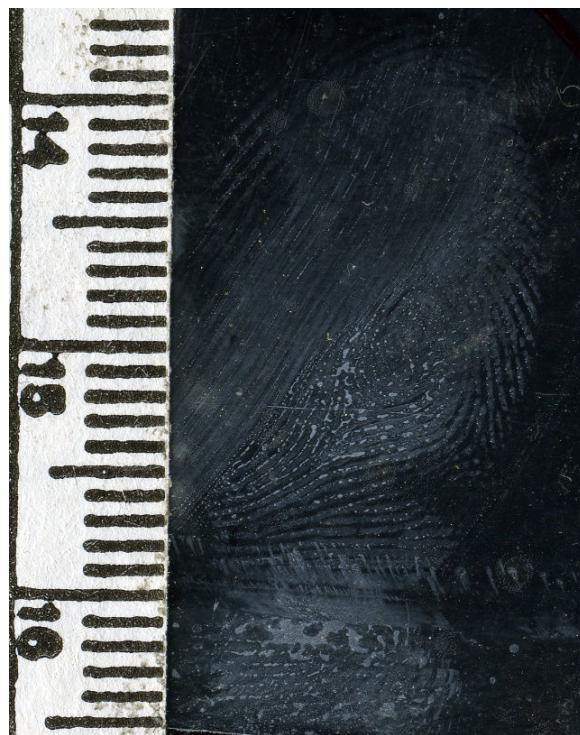
**Pressure distortion (PD) – distortion due to deposition pressure**
