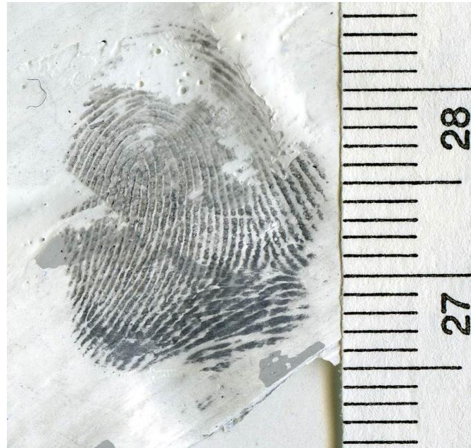
Example: distortion from areas of ridges disconnected by voids from writing on substrate (black powdered print)
