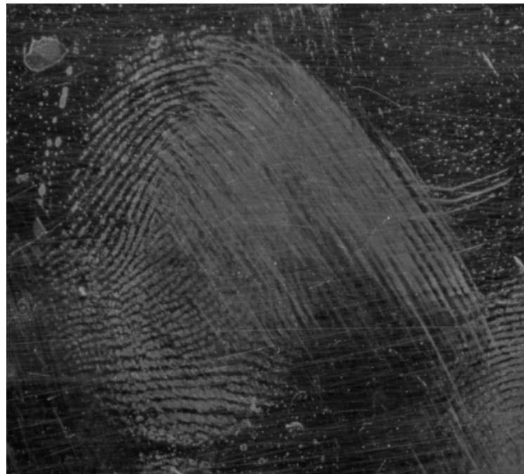
**Twisting (TW) – unnatural ridge flow due to torque**
