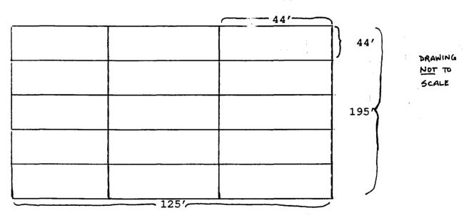
The sampling grid yields fifteen (15) boxes of which the center of each is sampled. This grid pattern can be integrated with those samples already obtained. It may be necessary to sample beyond the original grid in order to determine the full horizontal and vertical extent of contamination.
