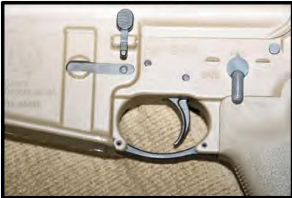
*(Photo of safety switch on 'FIRE' position)*
