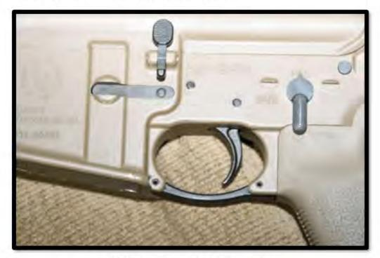
(Photo of safety switch on 'FIRE' position)
